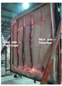
2. Exposed face of test specimen after the completion of the test
